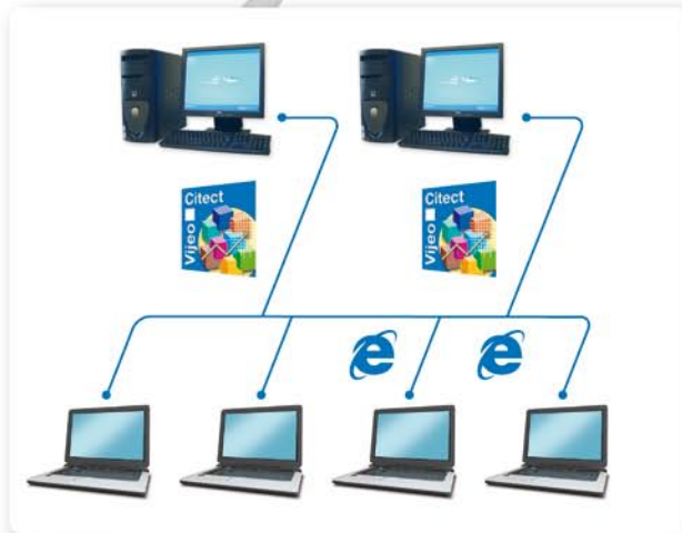
Redundant architecture with 2 servers and 2 Web clients
